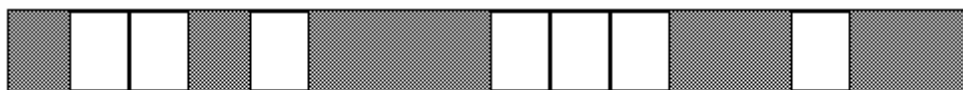
16 bits handles 16K of memory with the chunk (page) size of 1K
